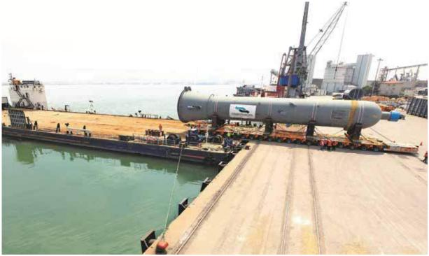
Hareket also specializes in load-out services. Our engineers and naval project team have extensive expertise in engineering and executing complicated load-outs of offshore modules, top sides, jackets and other types of heavy loads. These services for the offshore and modularization projects include, but are not limited to:
